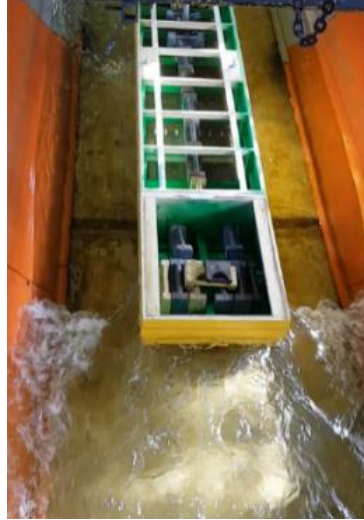
Figure 8. Resistance test in channel above the critical speed V_{CR} .
