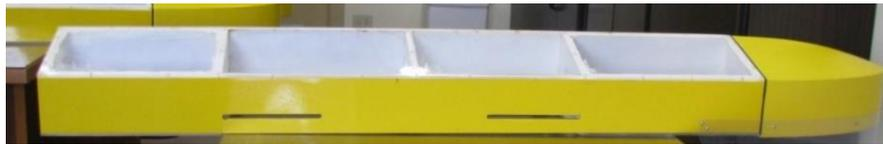
**Figure 3.** Monohedral hull geometry
