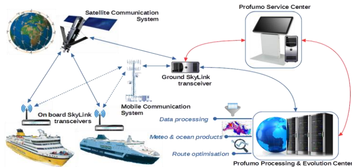
Figure 1. Overall PROFUMO Demonstrator system architecture.
