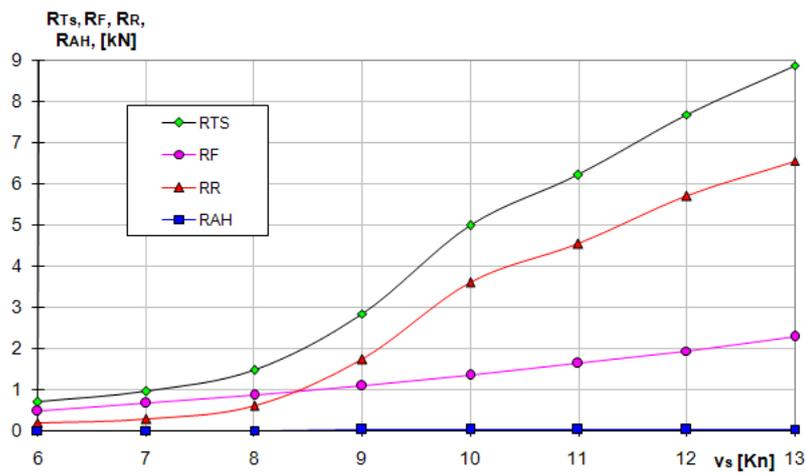
Figure 2. Total yacht resistance and its components
