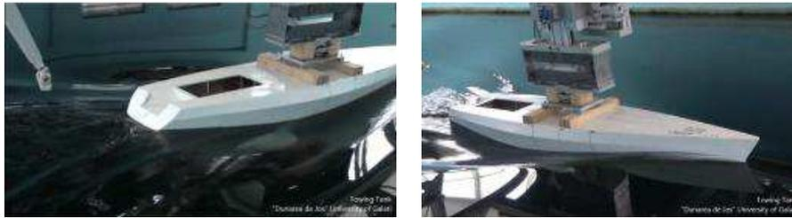
Figure 5. Hydrodynamic flow,  $\phi = 0^\circ$ ,  $v = 1.5$  m/s (full scale 9.22 Kn)
