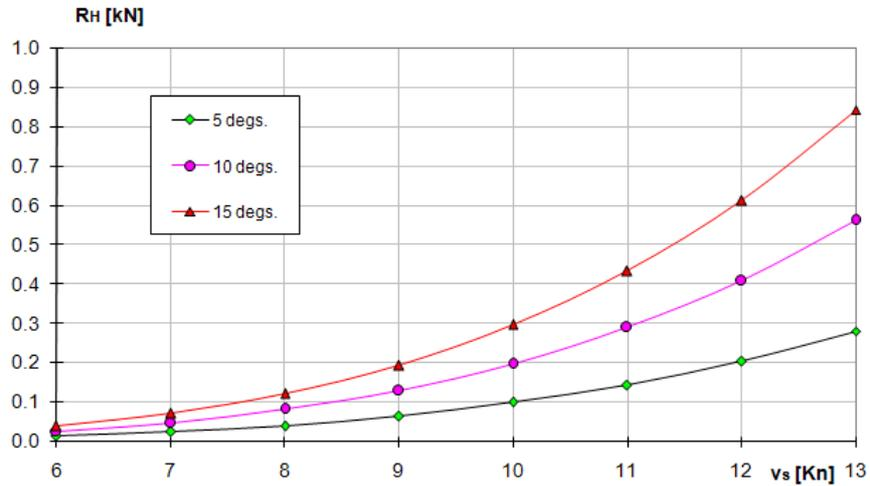
Figure 4. Heel resistance component of the yacht
