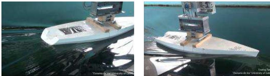
Figure 9. Hydrodynamic flow,  $\phi=15^\circ$ ,  $v=1.5$  m/s (full scale 9.22 Kn)
