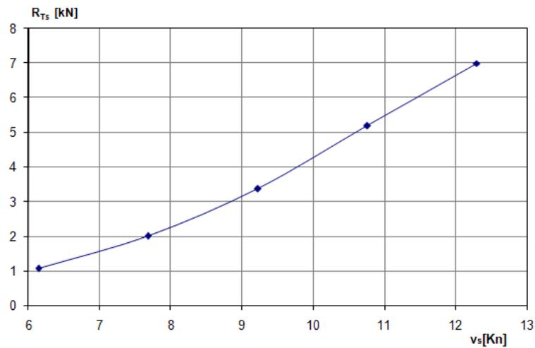
Figure 7. Full scale total yacht resistance (extrapolated)
