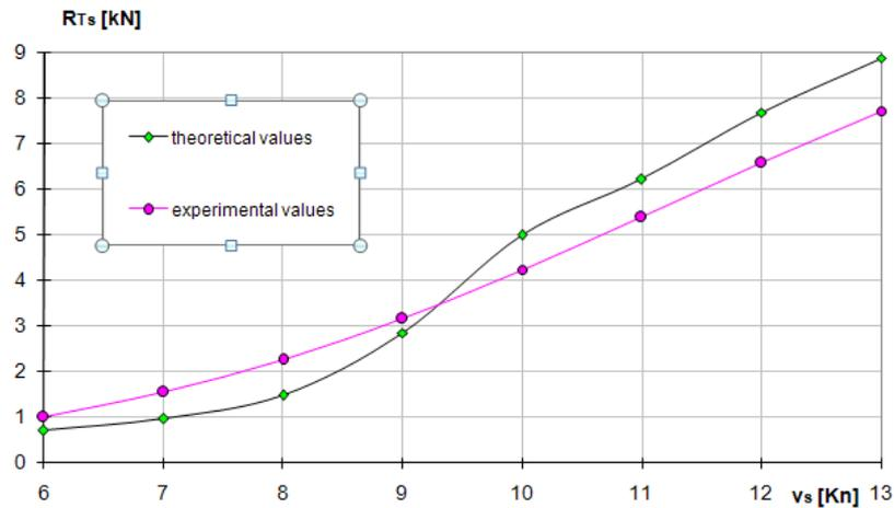
Figure 10. Theoretical and experimental total yacht resistance
