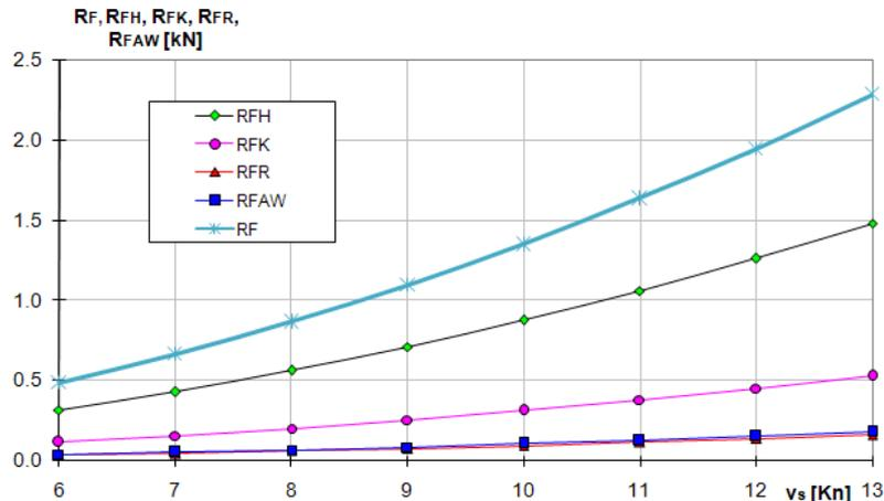
Figure 3. Frictional resistance of the hull with appendages and its components
