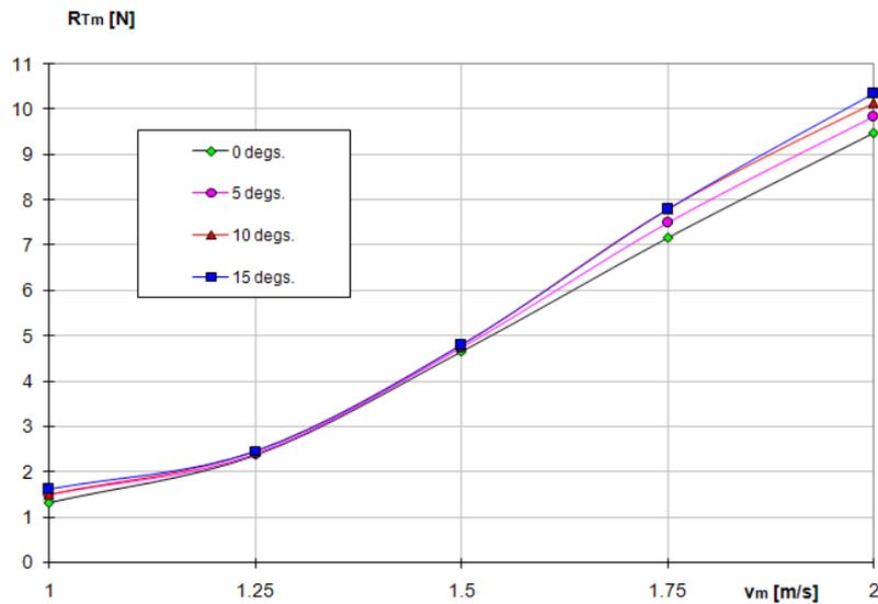
Figure 8. Heeling angle influence on the model resistance
