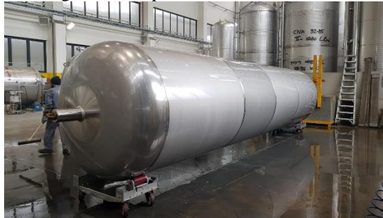
Figure 5. First liner built for hydroforming and testing (April 2018)
