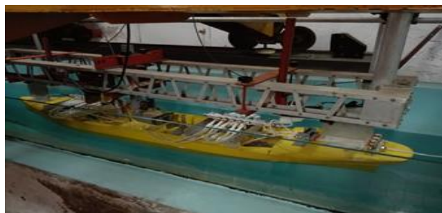
Figure 6. Hull assembled at the dynamometric carriage.
