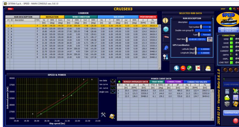
Figure 5: SPEED main console
