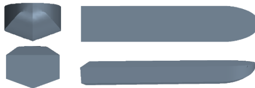
Figure 1. Geometry of the Fridsma hull.
