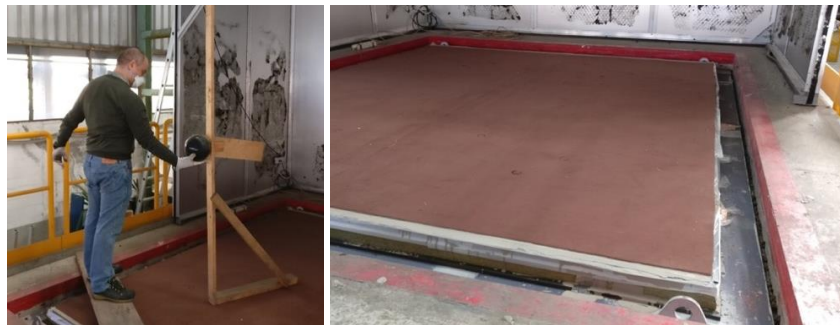
Figure 4. The heavy/soft normalized rubber ball dropped from 1 m (left) and the naval floor with laminated coating (right).
