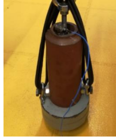
Figure 1. Impact hammer with inertial force estimation by shock accelerometer.
