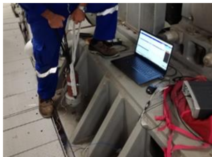
Figure 3. Application of artificial excitation generated by the inertial hammer on the diesel engine.
