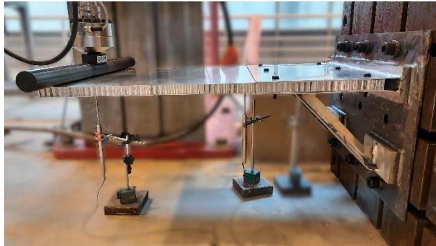
Figure 4. Experimental setup for full-scale testing of the AHS-based balcony overhang.
