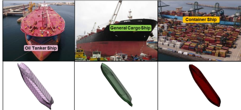
Figure 3. Panel discretization for the 3 ships.
