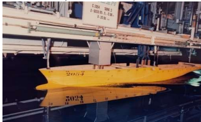
Figure 1. The generating hull model 2054 during the tests
