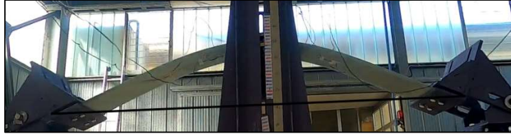
Figure 6. Impact no. 6 - Maximum deflection (380 mm) for G2, 20 mm, manufacturer “A” specimen (Image taken from a recorded video)
