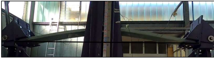
Figure 7. Impact no. 6 - Maximum deflection (180 mm) for G2, 40 mm, manufacturer “A” specimen (Image taken from a recorded video)
