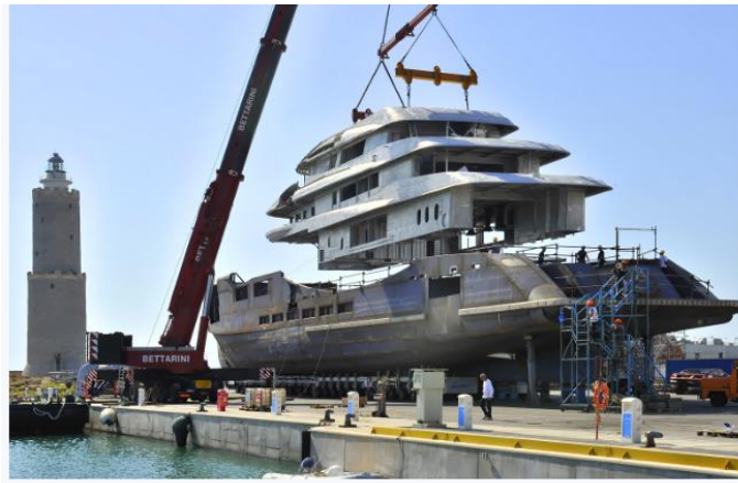
Figure 1. Welding steel hull to aluminium superstructure [8].
